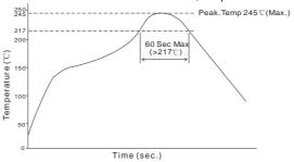
Note: The curve applies only to the hot air reflow soldering
